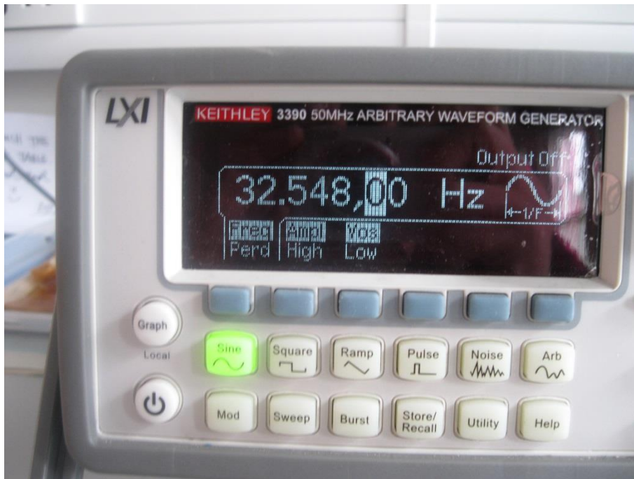
Figure 12: Digital meter showing frequency of waveform to nearest 0.0005 Hz
