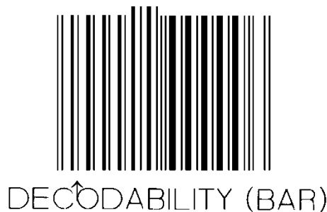
Figure 5.5.3.3.12 - 3 Calibration Symbol with Engineered Low Decodability Grade
