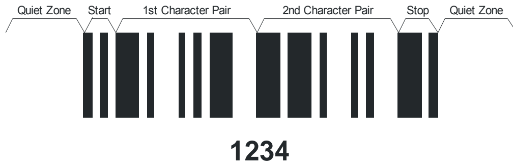
Figure 5.3.1.2.2 - 2 ITF-14 Symbol Inclusive of Quiet Zones
