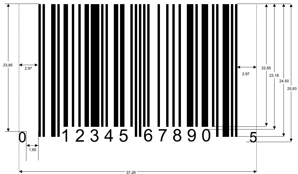
Figure 5.2.4.6 - 2 UPC-A Bar Code
