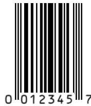
Figure 5.2.2.3.4 - 1 UPC-E Bar Code (Encoding 001234000057 by Zero-Suppression)
