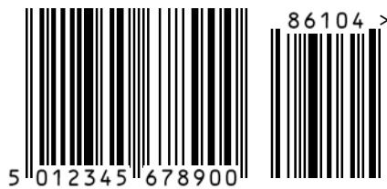
Figure 5.2.2.3.5.2 – 2 EAN-13 Bar Code with Five-Digit Add-On Symbol
