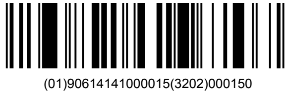
Figure 5.6.1.4.1 - 1 GS1 DataBar Expanded Bar Code
