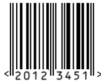
Figure 5.2.2.3.2 – 1 EAN-8 Bar Code
