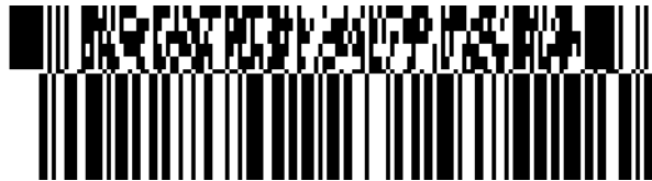
Figure 5.8.2 - 2 GS1-128 Composite Symbol with CC-C
