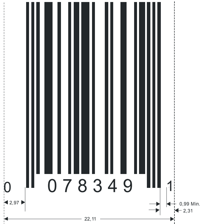
Figure 5.2.4.6 - 5 UPC-E Bar Code
