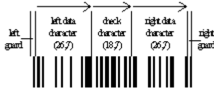
Figure 5.6.1.3 - 2 GS1 DataBar Limited Bar Code Structure
