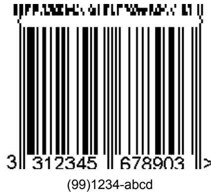
Figure 5.8.8 - 1 EAN-13 Symbol with a Four-Column CC-A Component
