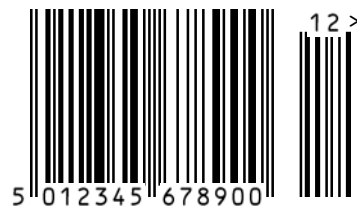
Figure 5.2.2.3.5.1 - 2 EAN-13 Bar Code with Two-Digit Add-On Symbol
