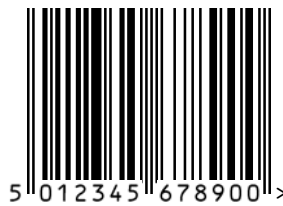
Figure 5.2.2.3.1 – 2 EAN-13 Bar Code
