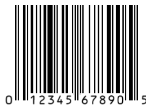
Figure 5.2.2.3.3 - 1 UPC-A Bar Code
