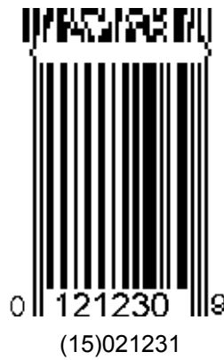
Figure 5.8.8 - 4 UPC-E Symbol with a Two-Column CC-A
