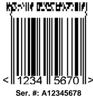
Figure 5.8.8 - 3 EAN-8 Symbol with a Three-Column CC-A
