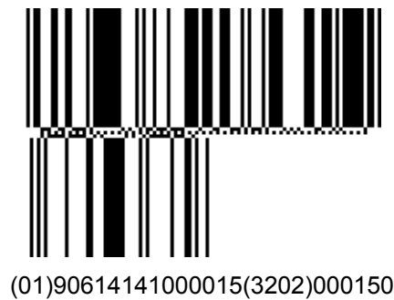
Figure 5.6.1.4.2 - 1: GS1 DataBar Expanded Stacked Bar Code
