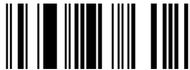
Figure 5.6.1.2.1 - 1 GS1 DataBar Omnidirectional Bar Code
