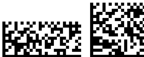
Figure 5.7.3.1 - 1 Rectangular and Square GS1 DataMatrix Symbols
