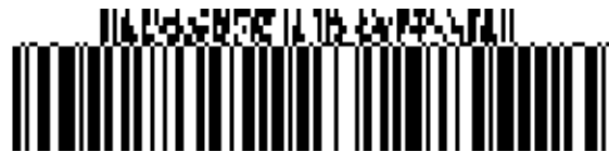
Figure 5.8.8 - 9 GS1-128 Symbol with a Four-Column CC-A
