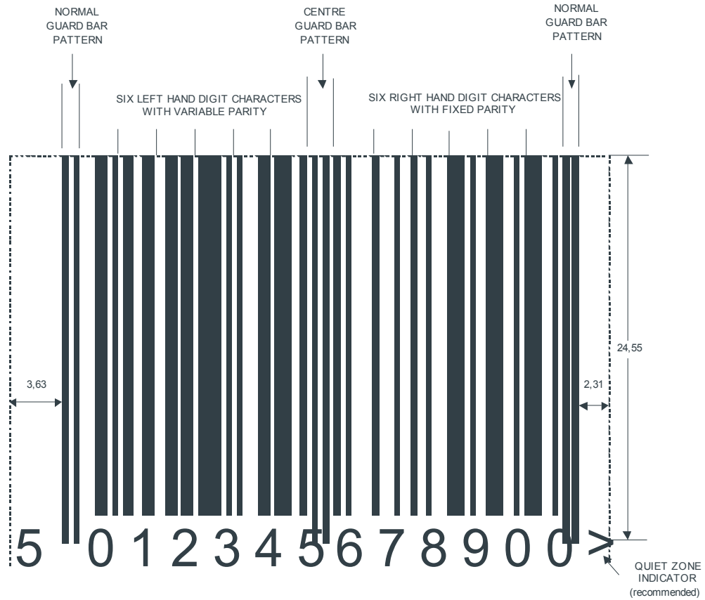
Figure 5.2.4.6 - 1 EAN-13 Bar Code
