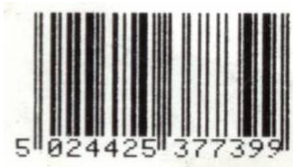
Figure 5.5.3.3.12 - 1 Symbol with Edge Determination Problem
