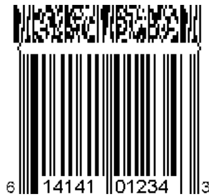
Figure 5.8.8 - 2 UPC-A Symbol with a Four-Column CC-B Component
