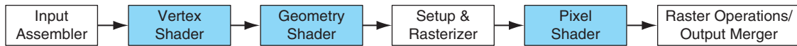
FIGURE C.2.3 Graphics logical pipeline. Programmable graphics shader stages are blue, and fixed-function blocks are white.
