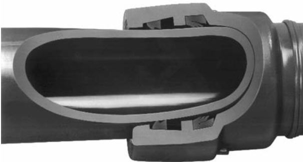
Section through Push-Fast assembled joint showing grab ring in taper and elastomeric seal.
