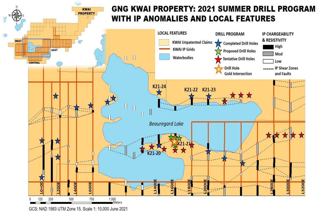
Figure 2 IP anomalies and drill holes at Beaugard Lake
