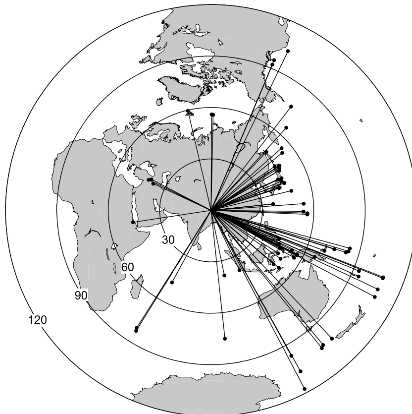
Figure 2. Azimuthal distribution of the teleseismic events used in this study. Epicentral distance from the centre of the seismic array is shown with concentric circles with degrees on the great circle.
