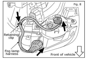
8. Plug the fog lamp harness into the connector at the back of the fog lamp. Plug the other end of the harness into the pre-wire vehicle harness connector.
