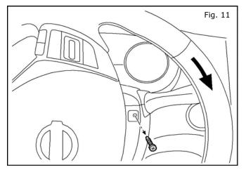
11. Rotate the steering wheel clockwise to access the right steering column cover screw. Remove one (1) phillips head screw.
