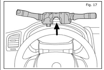
17. Remove the combination switch by lifting up and out of steering column.
