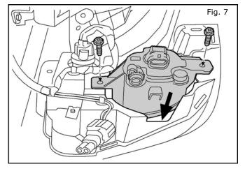
7. Install fog lamp assembly into fascia and secure with two (2) 10mm self-tapping bolts.
