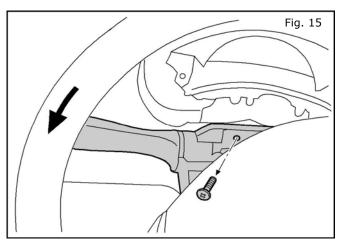
15. Rotate the steering wheel counter clockwise and remove one (1) combination switch mounting screw on the left.
