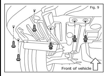
9. Carefully press the lower cover panel back into position. **Reinstall** the lower cover using the three (3) phillips head screws and three (3) retaining clips.
