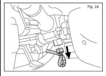
16. Locate the combination switch connector plug on the underside of the steering column and disconnect.
