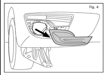
4. Carefully pry off the passenger side fog lamp finisher cover by depressing the retaining tabs on the inside of the fascia. Push the finisher cover outward from behind.
