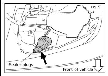
5. Locate the pre-wire harness connector inside the lower edge of the fascia.
