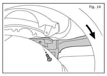
14. With the steering wheel turned to the right, use a phillips head screwdriver to remove one (1) combination switch mounting screw.
