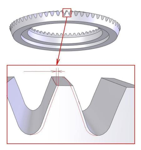
Lead crowning is used with profile crowning for reduction of sensitivity for misalignments and other errors. But more crowning reduces the gear life. Picture below shows both: lead and profile crowning.
