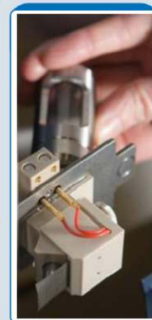
Spray head with matrix reservoir
