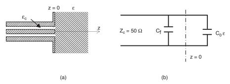
**FIGURE P1.11** Coaxial probe terminated to lossy medium with complex permittivity  $\varepsilon$ : (*a*) schematic of the probe; (*b*) equivalent circuit model.
