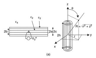
FIGURE P1.15a Insulated dipole in lossy medium.
