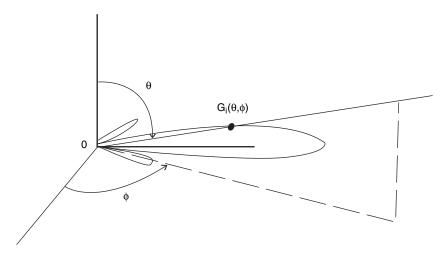
FIGURE 1.5 Radiation diagram of an antenna.
