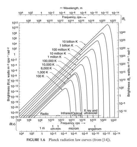
According to the Rayleigh–Jeans law, the brightness varies inversely as the square of the wavelength. On a log-log graph this relation appears as a straight line of negative slope. It coincides with Planck's law for the same temperature at long wavelengths. At short wavelengths, however, the brightness predicted by the Rayleigh–Jeans law would increase without limit, whereas the actual brightness reaches a peak and then decreases with decreasing wavelength, as predicted by Planck's law.
