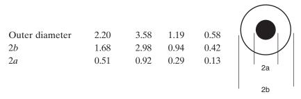
The dielectric is Teflon ( $\varepsilon_c = 2.1$  and tan  $\delta = 0.0001$ ). At 915 MHz and 2.4 GHz, find the dielectric, conductive, and total loss if the conductors are copper.
