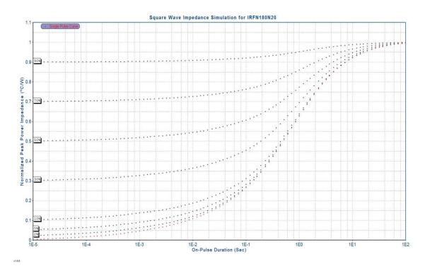
Once an approximate set of parameters has been determined, the dynamic thermal model can be exercised to predict the actual junction temperature excursion during the proposed power pulse:
