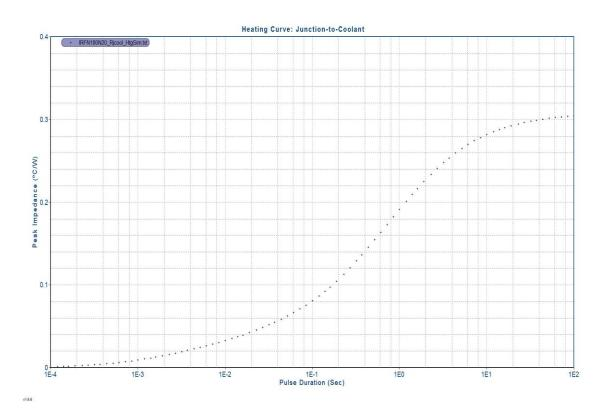
This heating curve is referenced to the coolant temperature, not case temperature, since the coolant is the essential reference for the determination of the device junction temperature. Using a dynamic thermal model that embodies this transient response, the predicted device impedance response to any cyclic heating waveform can be determined and expressed in a plot as a function of the on-power duty cycle.
