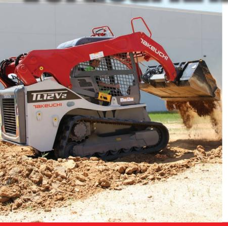
Vertical arm machines have minimal change in the loaders center of gravity because the load is kept closer to the machine throughout the arm path. They are ideal for loading trucks and hoppers with high sides and generally provide better reach at dump height.
