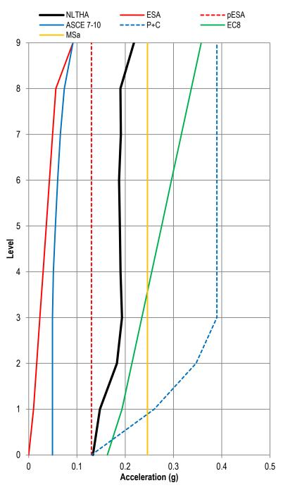
**Figure 10. Building G. Diaphragm acceleration (a) envelopes and (b) low-pass filtered envelopes.** Further discussion on the design and modelling methodology can be found in Section A.7.
