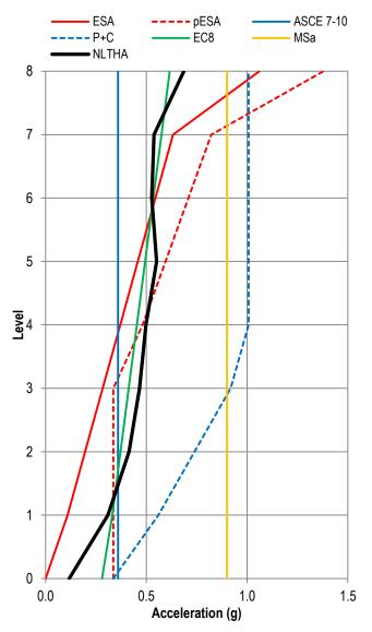
Figure 17. Building F. Diaphragm acceleration low-pass filtered envelopes.
