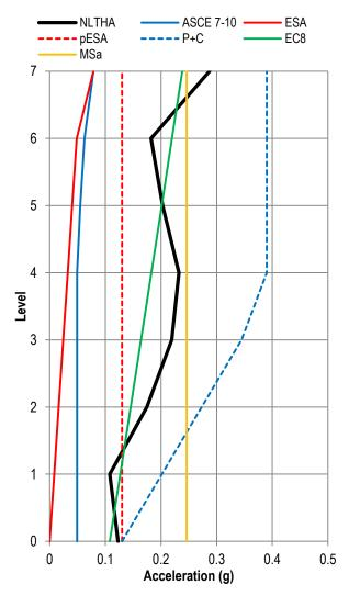
Figure 16. Building E. Diaphragm acceleration (a) envelopes and (b) low-pass filtered envelopes.
