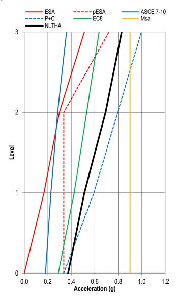
Figure 13. Building B. Diaphragm acceleration low-pass filtered envelopes.
