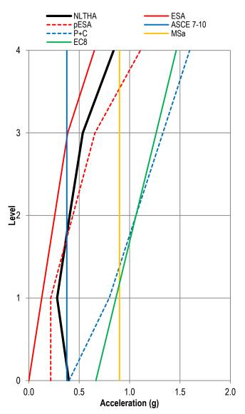
Figure 14. Building C. Diaphragm acceleration low-pass filtered envelopes.
