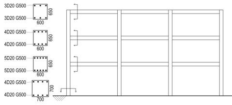
Figure 23. Building B. Sketch of the structural solution.
