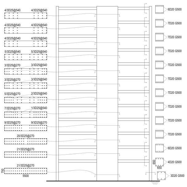
Figure 28. Building D. Sketch of the structural solution.
