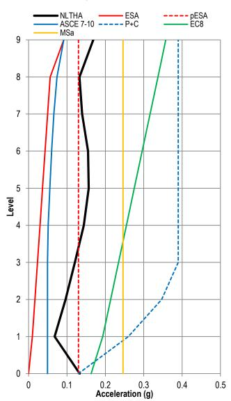
Figure 18. Building G. Diaphragm acceleration low-pass filtered envelopes.
