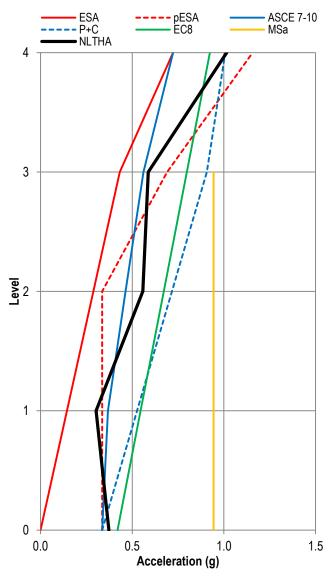
Figure 12. Building A. Diaphragm acceleration low-pass filtered envelopes.
