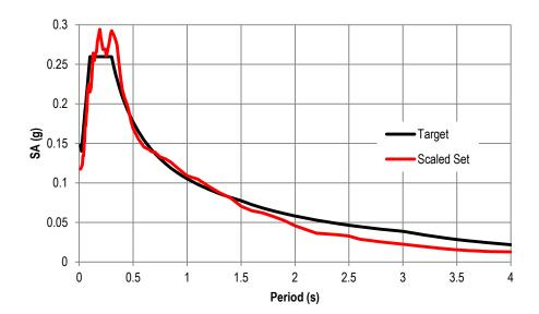
Figure 1. Auckland record set average spectrum (scaled at  $T_1 = 1.0s$ ).
