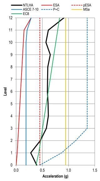
Figure 15. Building D. Diaphragm acceleration low-pass filtered envelopes.
