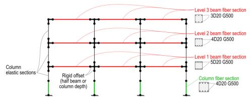
Figure 24. Building B. Sketch of the nonlinear model.
