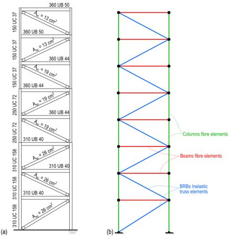
Figure 32. Building F. Sketches of (a) the structural solution and (b) the nonlinear model.
