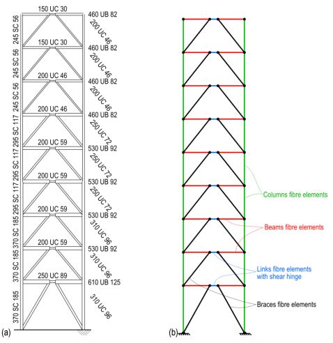
Figure 34. Building G. Sketches of (a) the structural solution and (b) the nonlinear model.
