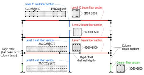
Figure 11. Building D. Sketch of the nonlinear model.
