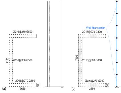
Figure 30. Building E. Sketches of (a) the structural solution and (b) the nonlinear model.
