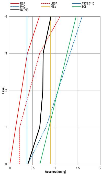
Figure 6. Building C. Diaphragm acceleration envelopes.
