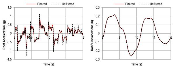
Figure 11. Building D, EQ01 (a) acceleration and (b) displacement response (filtered and unfiltered).
