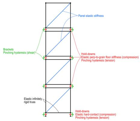
Figure 21. Building A. Sketch of the nonlinear model.
