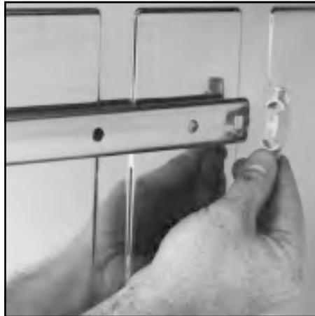
Fig. 5-3 To remove the Rail, disengage the End Cap by applying outward pressure to the Cap's top tab, unclipping it from the Rail. Then slide the Rail out from the Guide Rollers.
