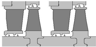
Fig. 5 Turbine stage configuration overview
