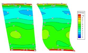
Fig. 20 Stage outlet entropy contours (left: original, right: optimal)
