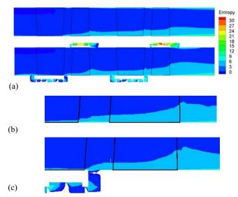
Fig. 7 Meridional view of entropy contours without leakage (top of a), with leakage (bottom of a), close-up of first stage hub without leakage (b) and close-up of first stage hub with leakage (c)
