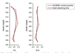
Fig. 14 Tendency of the optimum blade stacking line change of the first and the second stage rotor blades
