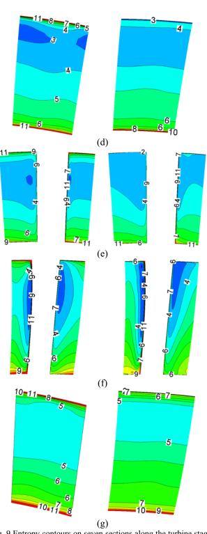
Fig. 9 Entropy contours on seven sections along the turbine stages (left: without leakage, right: with leakage)
