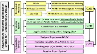
Fig. 1 Aerodynamic optimization design system
