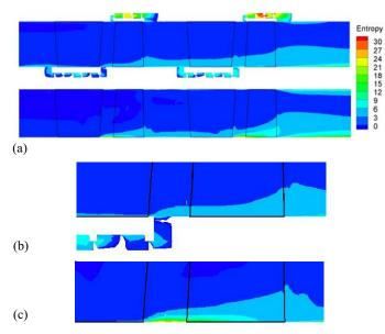
Fig. 12 Meridional view of entropy contours with full mesh leakage calculation (top of a), with simple leakage calculation (bottom of a), close-up of first stage hub with full mesh leakage calculation (b) and close-up of first stage hub with simple leakage calculation (c)
