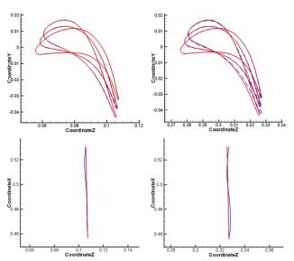
Fig. 18 Blade control sections and trailing edges (left:1st rotor, right: second rotor; red: original, blue: optimal)
