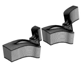
Fig. 10 CFD mesh of the turbine stages
