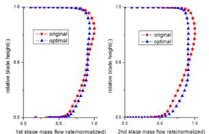
Fig. 19 Mass-flow distributions (left:1st rotor, right: second rotor; red: original, blue: optimal)
