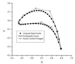
Fig. 2 Rotor blade hub profile represented by NURBS
