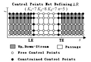
Fig. 4 NURBS control point net of the radial coordinate change function
