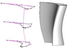
Fig. 3 Leaned rotor blade made by NURBS techniques
