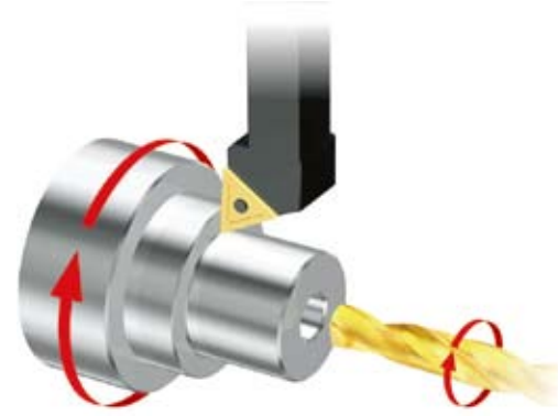
Differential velocity cutting by revolving tools In multiple cutting of inner and outer diameters, the optimum cutting speed can be obtained by controlling the revolving tool speed. A small-diameter drill is rotated in the forward direction to increase the relative speed between the drill and the workpiece, while a large-diameter drill is rotated in the reverse direction to decrease the relative speed.
