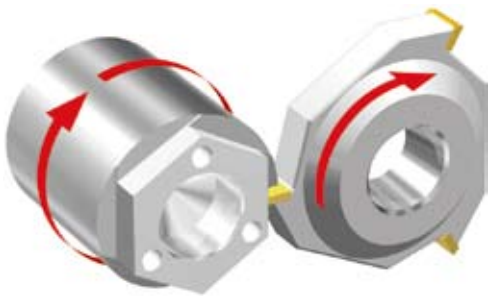
Polygon machining (Optional) Synchronizing the revolving tool speed with the spindle speed at two times permits polygon machining, such as two-, four- and six-sided machining, with a polygon cutter.
