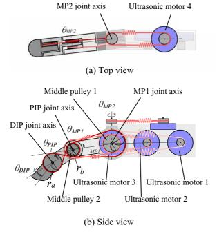
Fig. 3 Outline of driving mechanism of fingers
