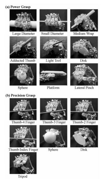
Fig. 11 Result of grasping experiment based on Cutkosky's taxonomy [12]
