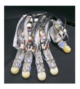
Fig. 6 Developed five-fingered robot hand
