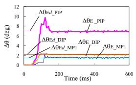
Fig. 9 Response of  $\Delta\theta_{\rm E}$  in force control experiment
