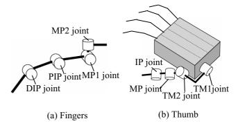
Fig. 2 Arrangement of DOF
