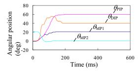
Fig. 7 Step response of robot index finger
