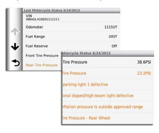
With The **Motorcycle status** page riders can view vehicle information fed to the Navigator V via the LIN bus when off the bike. It allows a quick glance of the most recent snap shot from the bike.
