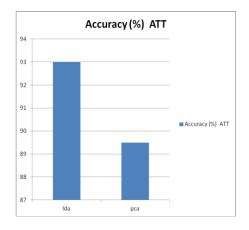
Fig. 3. Accuracy PCA and LDA using ATT database
