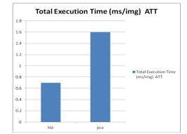
Fig. 6. Total execution time taken in millisecond for each image(ATT)
