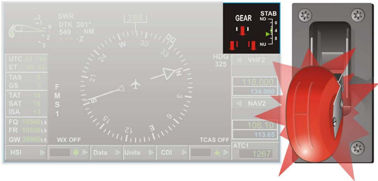
FIGURE 02-32-30-00 HSI WINDOW, GEAR IN TRANSIT WITH TOO LONG EXTENSION TIME
