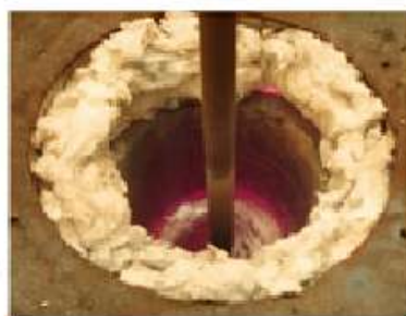
Fig 2 Stirring by motorized stirrer
