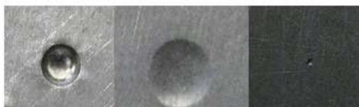
Fig 8 Indentation of Rockwell, Brinell and Vickers hardness test respectively
