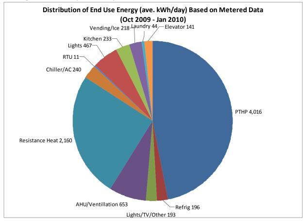
Figure 4. Monthly Electricity End-Use for the Four Metered Months (Combined)
