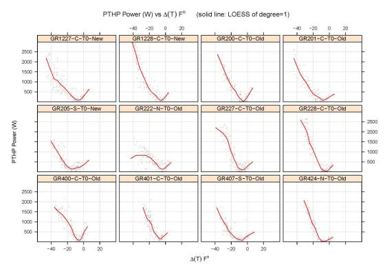
Figure 5. PHTP Average Power Consumption as Function of Average Daily Difference in Outdoor and Return Air Temperatures
