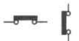
INTERLOCK-- NORMALLY CLOSED
