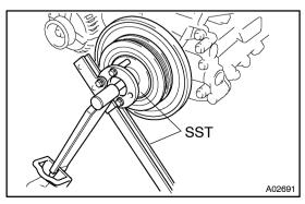
18. TIGHTEN CRANKSHAFT PULLEY BOLT
