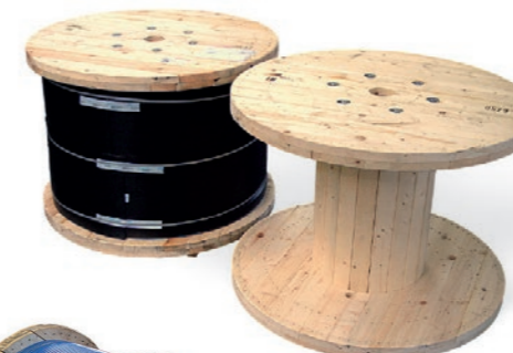
XJ-Wooden Reels ø100 x 65 cm capacity according to rope diameter from 1000 m HRS (ø 16 mm) or 1132 kg reel weight up to 4100 m HRS (ø 8 mm) or 1118 kg reel weight
