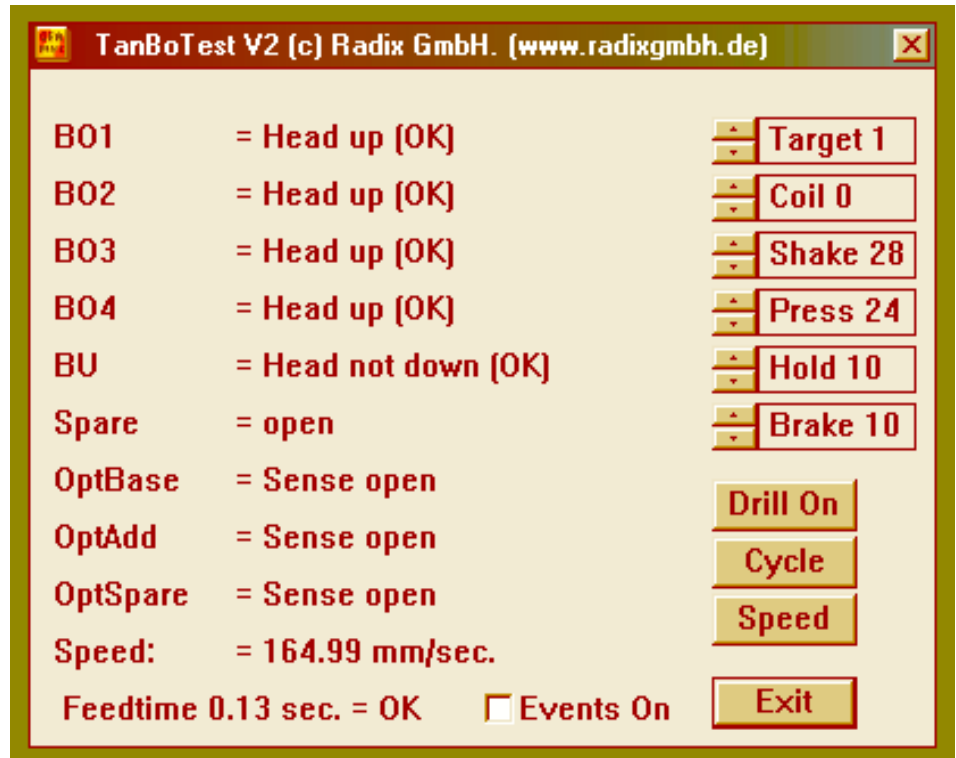
Figure 1. The TanBoTest utility tests the various microswitches and determines the operating parameters to be stored in the configuration file.
