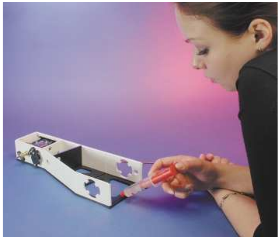
Figure 2. In a single motion, draw out a line of glue along the full length of the joint.
