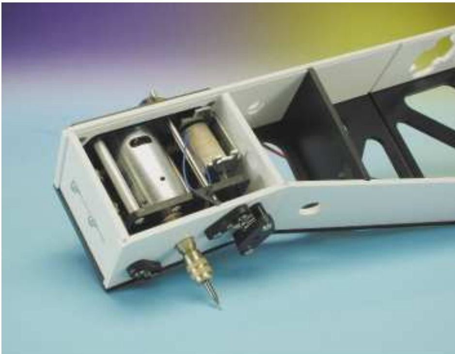
Figure 3. Partially-glued tool arm with drill motor and solenoid already fitted.
