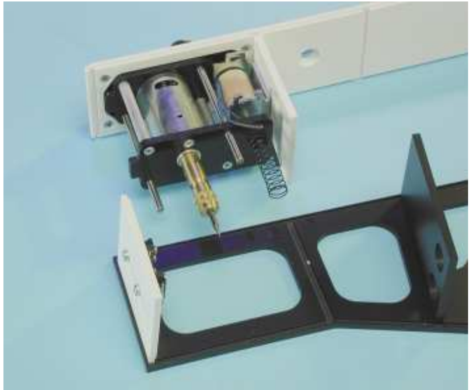
Figure 8. Fitting the drill lift assembly.
