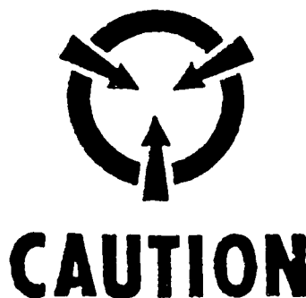
FIGURE 9.1: MIL-STD-129 SENSITIVE ELECTRONIC DEVICE SYMBOL
