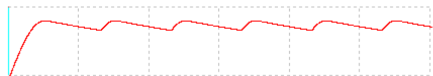
Figure 3.8: Full wave rectified Output Signal with filter
