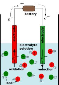
electrode and pump electrons into the other. This process forces current to flow, and so the battery becomes a source of electricity. In an electrolytic cell, we supply the power driving the current with an external battery and use that to force a chemical reaction to occur.
