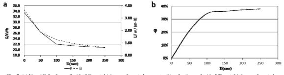
Fig. 7. (a) U and E for the roof with different thickness of aerated concrete; (b)  $\varphi$  for the roof with different thickness of aerated concrete. From Fig.7, the reasonable thickness of aerated concrete layer for the roof is 100-150mm, the heat transfer coefficient of roof is between 0.94 w / (m· K) and 1.25 w / (m· K). The energy saving rate limit value of the aerated concrete roof is estimated below 40%.
