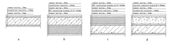
Fig. 2. (a) Contrast roof; (b) Light insulation roofing for inside; (c) Light insulation roofing for outside; (d) Heavy insulation roofing.
