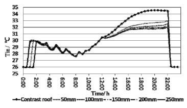
Fig. 6. Indoor hourly temperature for different aerated concrete layer of roof.
