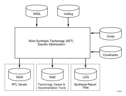
XST takes in Verilog and/or VHDL files to be parsed and synthesized, "Cores" which are pre-built circuits designed by Xilinx, and "Constraints" (an XCF file). In this lab we don't supply any cores or constraints to xst.
