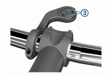
7 Press down slightly and turn the Edge device clockwise until it locks into place.
