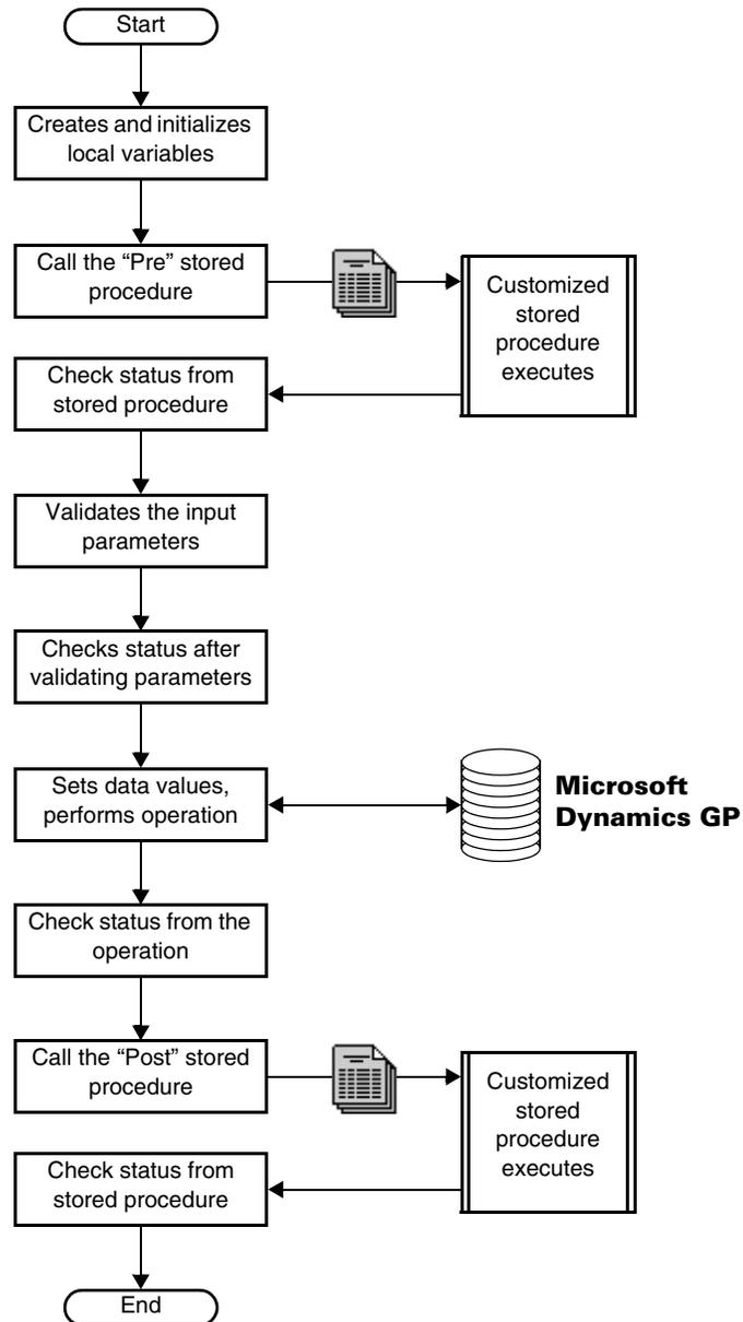
Notice how the business object validates data parameters, adds default values, and performs a status check after each event. The business object uses status checks to handle errors. When a status check detects an error, it immediately stops the stored procedure, initiates a rollback of the transaction, and returns an error message to the caller.
