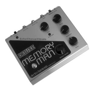
This model is based on the Electro-Harmonix Deluxe Memoryman. This pedal uses the "bucket brigade" electronics of other analog echoes, and adds a chorus circuit. This adjustable chorus is applied to the echoes only, leaving the direct sound unaffected.
