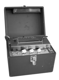
The classic 1963 Maestro EP-1 was the first of a series of "Echoplex" designs distributed by the company, and made by Harris-Teller in Chicago. As touted in a Maestro advertisement, the Echoplex's "...special effects range all the way from a controlled high speed reverberation to a full, throbbing echo"!
