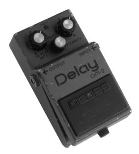
Analog echo units like the DM-2 were designed as improvements over the tape echoes that came before them, using "bucket brigade" electronics to give guitarists echo units that were more reliable than the tape-based delays, with the added advantage of a low power circuit that can be run on batteries.
