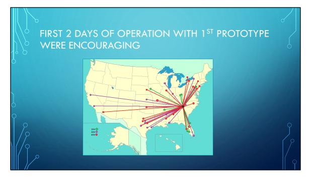
In the first two days of testing with the original lightbulb antenna, a number of QSOs, some out to 2000 miles, were completed on 40M, 30M and 20M. This was encouraging, so a decision was made to continue development.
