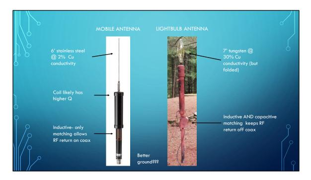
Here is a picture of a popular mobile antenna with a 6' stainless steel whip next to version 4 of the lightbulb antenna. The are very similar. But remember, the lightbulb contains a better radiator than stainless steel and this difference likely makes the lightbulb antenna perform better than one would think it should.
