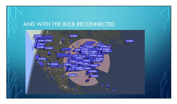
For the next test, I then put the lightbulb back into the antenna, retuned, and transmitted for another 5 minutes. Once again, the original distant stations were reporting my signal. It appears that success of the antenna is due to the big lightbulb.
