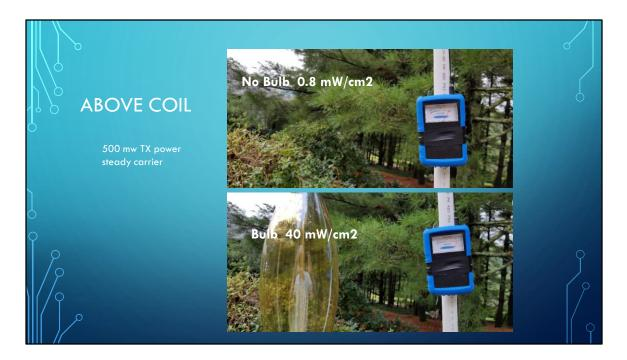
From the area of the lightbulb, very little current is detected when the lightbulb is removed from the circuit. When the lightbulb is in place, the radiated energy pegs the field strength meter at 40milliwatts/cm2.
