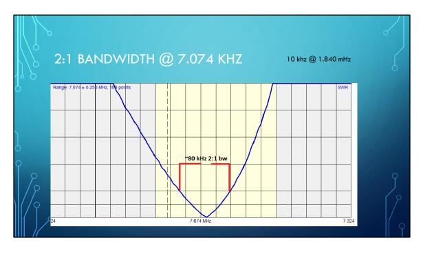
The 2:1 bandwidth looks pretty good on the antenna. It is not really wide which would suggest a poor quality antenna. On 40M the 2:1 bandwidth was about 80 kHz and this dropped to 10KHz on 160M. So attention to tuning of the antenna when doing large within-band shifts in frequency is important.
