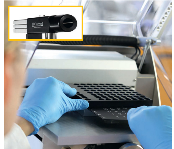
Figure 2: Autosampler with purge function - a purge chamber is continuously purged with helium before the sample is mechanically or manually fed to the combustion by the slider.
