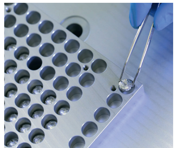
Figure 4: Sample weighing in tin foil (picture on the left) and placing samples in the sample tray until sample feeding in the autosampler (picture on the right).
