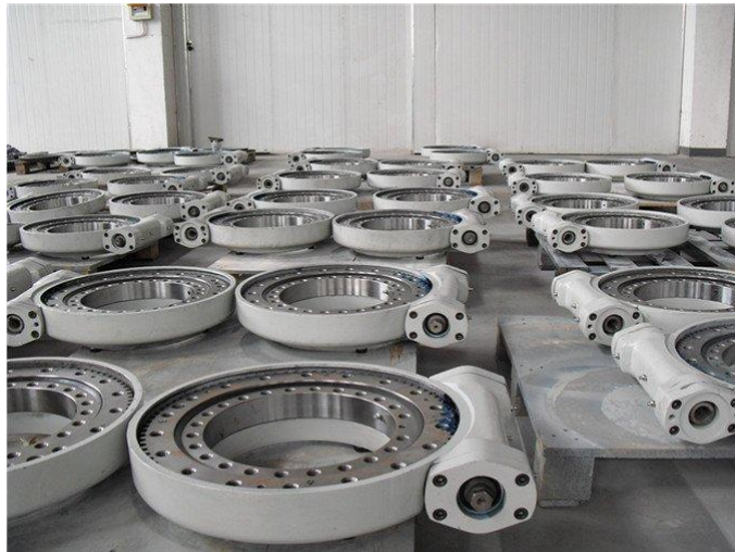
73 kg slewing drives begin assembled at Beijing Titanhorse Industry and Trading
