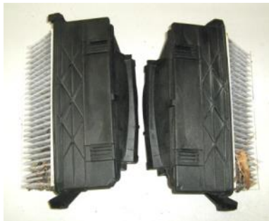
Picture 4: Contaminated air filters
