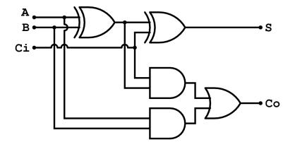
Figure 2.13: Circuit implementing a full adder
