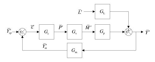
For the feedback control loop above the overall transfer functions between the output  $\overline{Y}'$  and the set point & disturbance are:
