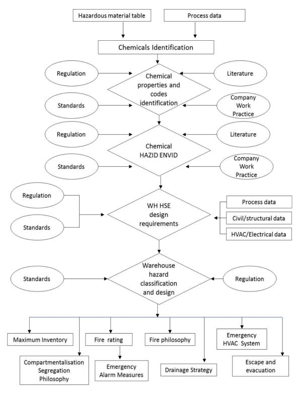
Figure 1: Warehouse safe design flow-chart
