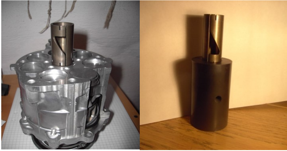
Figure 3: Illustration of the piston expander with a single rotating valve
