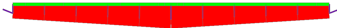
Figure 68 – Extrude view of the rib as composite beam. Slab in green, steel beam in red, stiff elements in purple.
