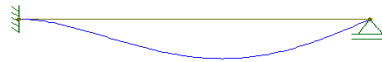
Figure 104 - Top view of the bridge's approximately deformed shape, when wind is applied.
