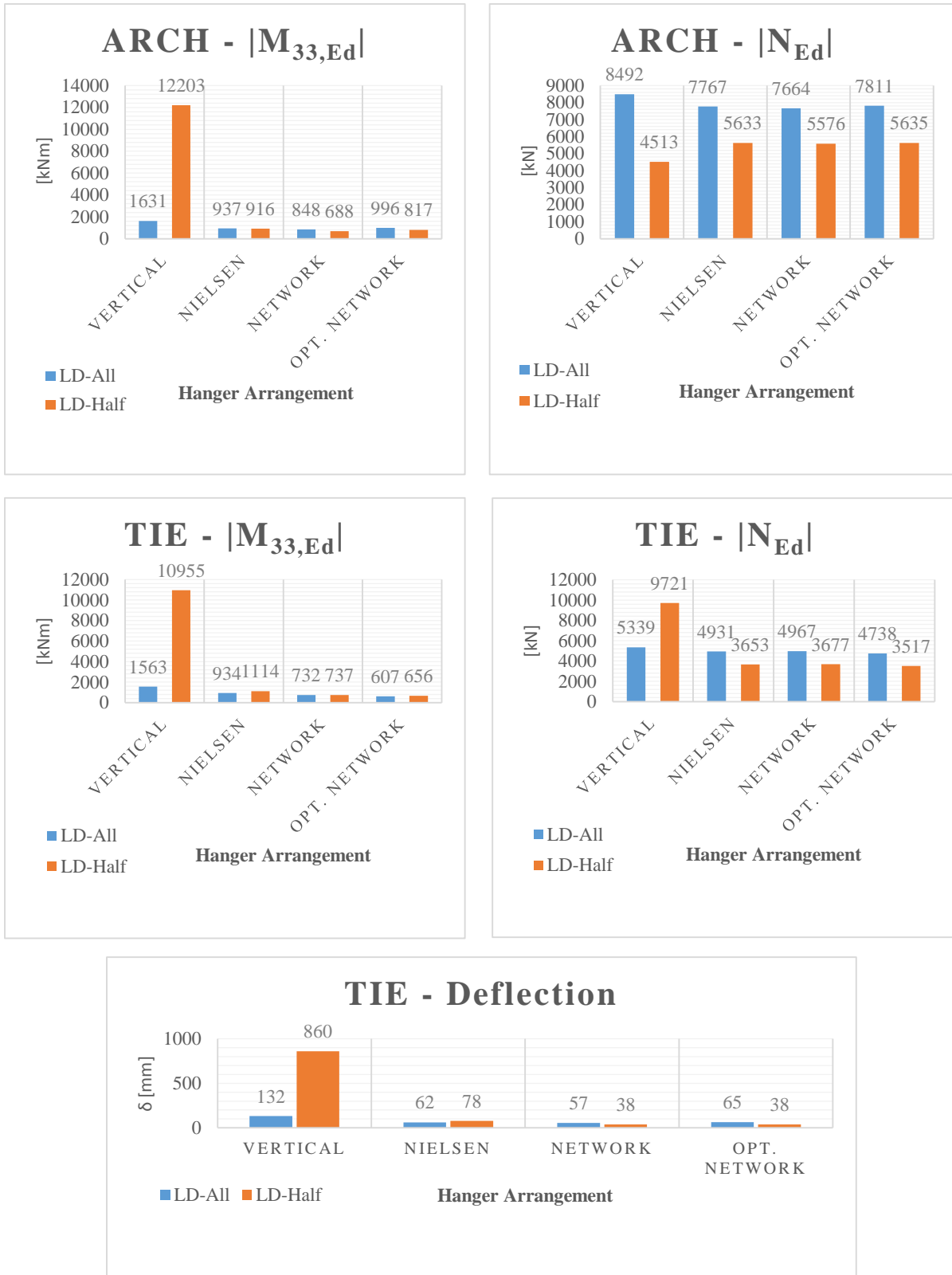
Figure 124 – Highest axial forces and bending moments in the arch and ties for the Live Load LM4 applied on all or half deck span.
