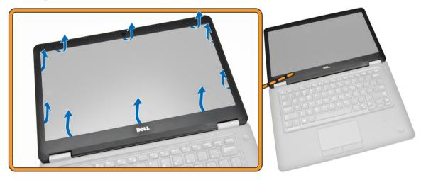
4 Remove the display bezel from the display assembly.
