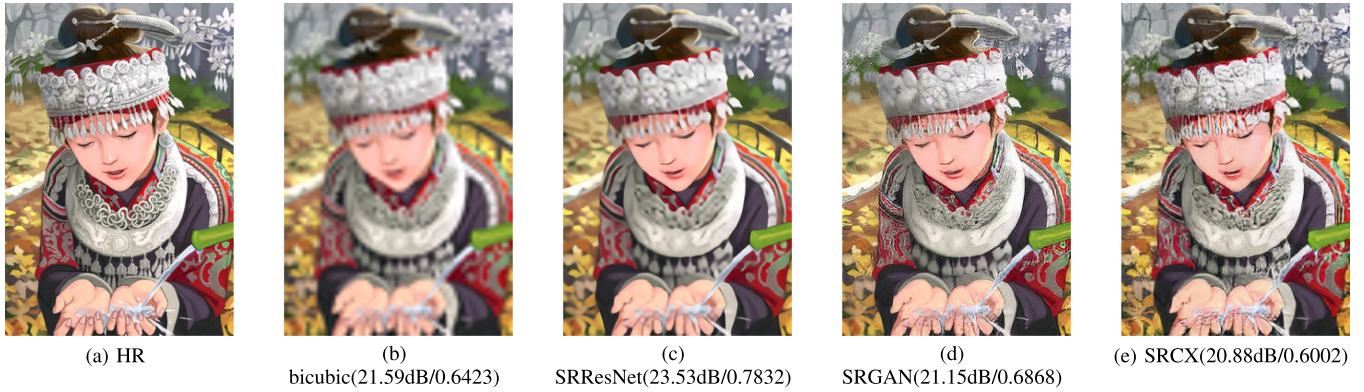
Fig. 12. Visual comparisons between the MSE, MSE + GAN and MAE +GAN + Contextual Loss (The authors of [68] and [116] released their results.) We can see that the perceptual loss leads to a lower PSNR/SSIM but a better visual quality.
