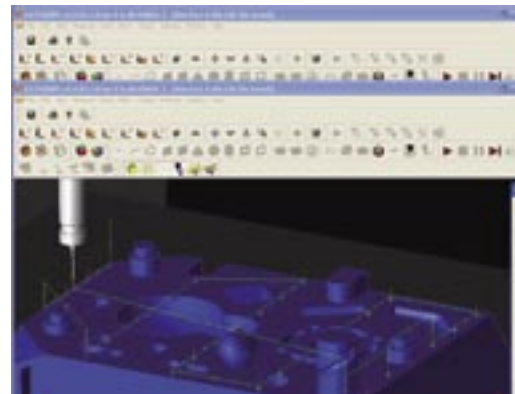
Interference check function prevents collisions
