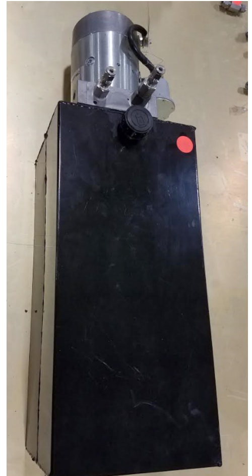
DC Power Unit
