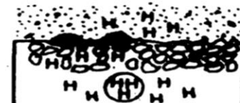
Hydrogen induced cracking
