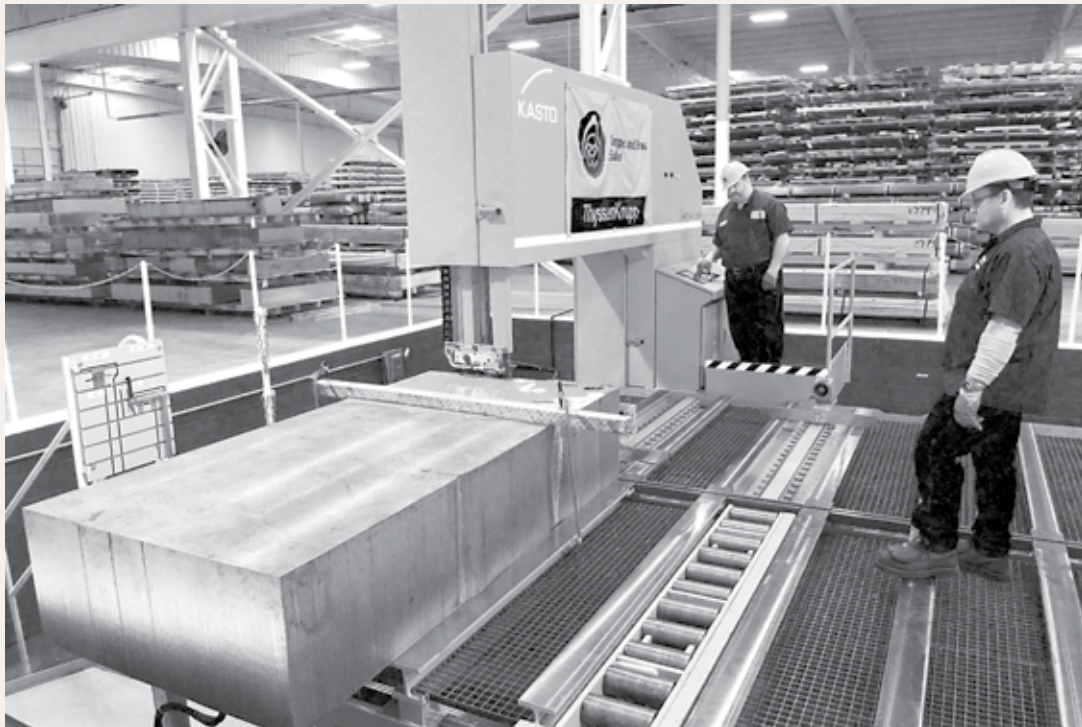
Heavy plate sawing to tight tolerances is a specialty at Copper and Brass Sales.
