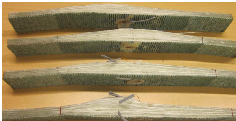
Figure 33 Tension failure in DGM.
