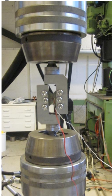
Figure 39 Shear test set up.
