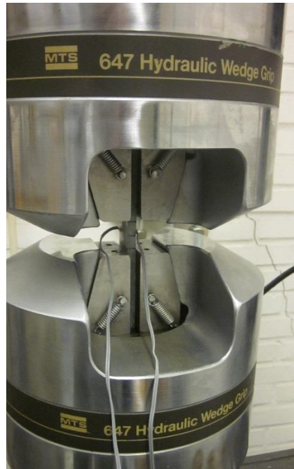
Figure 35 Compressive test set up.
