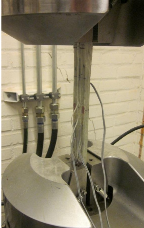
Figure 31 Tension test set up.
